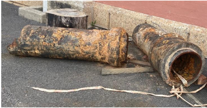
Left: Cast iron water pipes near Molteno reservoir. Right: The teak pipe in the City Hall collection.
